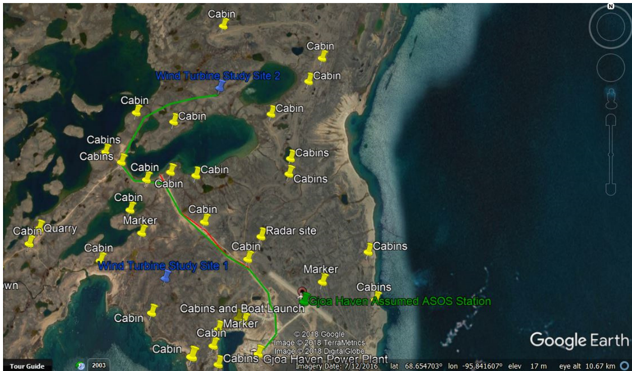
Figure 12 – Potential wind turbine sites near Gjoa Haven. Site #1 is low confidence due to shadow flicker. Site #2 is higher confidence but would still need a VOR waiver from Nav Canada.
